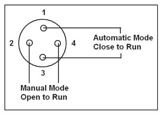
between pins 2 and 4 in interface connector and **AUTOMATIC/MANUAL Switch** should be set in **MANUAL** position. When external switch opens, Feeder will run.
