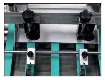
4. Rear Media Support Guide is adjustable to accommodate a wide variety of media. A knob [1] is provided to move Rear Guide front to back. Two thumbscrews [2] permit Guide to tilt and entire assembly [3] can be moved right to left. Position Guide so media is held up and against Separators. NOTE: Single sheets require more uplift than thick media and envelopes. A little experimentation will yield the best setup for each type of media.
