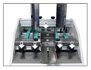
Position of Separator with respect to Feed Belts is determined by thickness of media you feed. If media is less than 1/8" (3.175 mm) thick, then Separators should be positioned between Center Belt and two Belts on either side (*as shown*). Separator should be adjusted to apply a light amount of pressure to force media between Belts.
