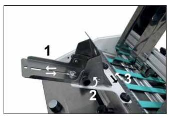
In addition to above, a Wide Media Plate is supplied to support wider media. It mounts in two slots in Rear Guide (*as shown*).
