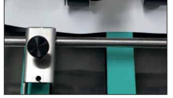
If feeding media over 1/8" (3.175 mm) and up to 1/2" (12.7 mm), Separators should be placed over Belts and adjusted so piece being fed clears, but next piece is held back.
